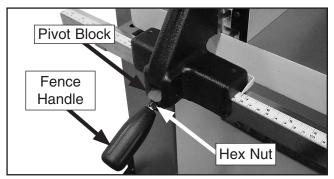
Figure 4. Fence handle components.
